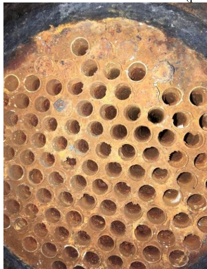
Рис. 1. Deposits of hardness salts in the heater of hot water supply
